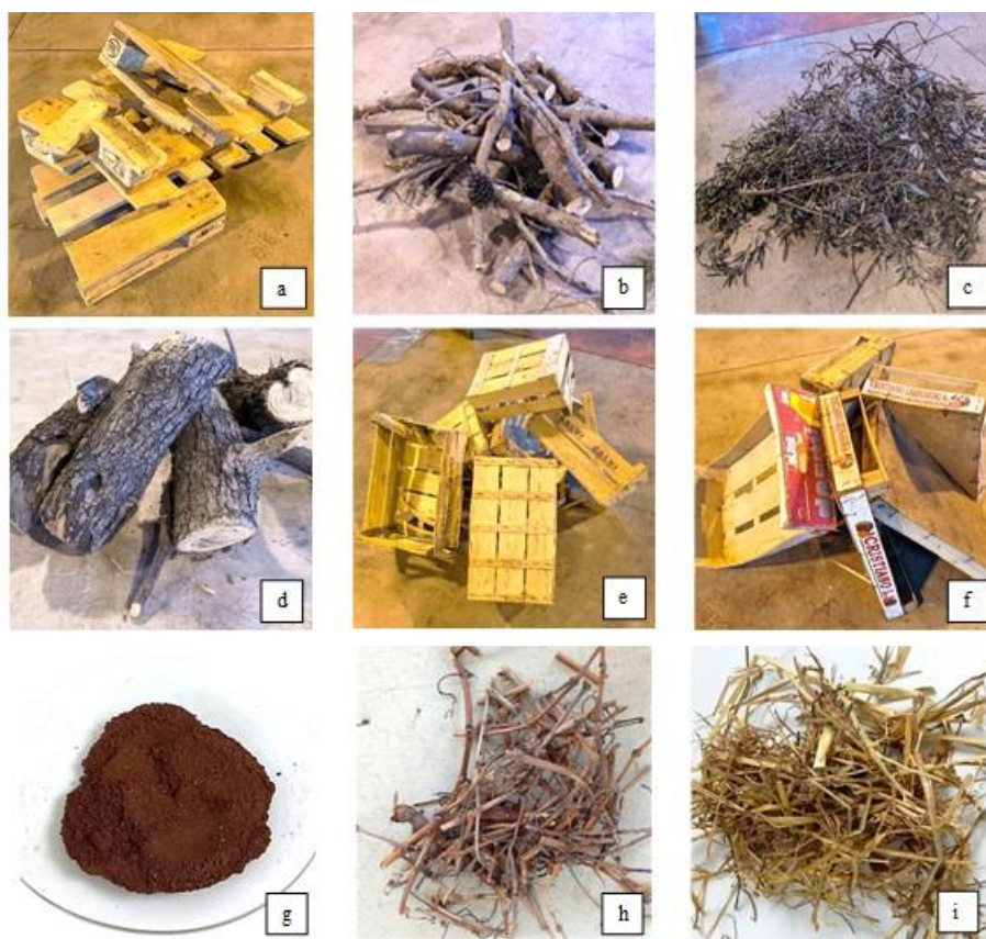
Fig. 1 – Biomasse tal quali: a) pallet, b) pino in tronchi, c) ulivo in ramaglie, d) ulivo in tronchi, e) cassette della frutta in legno, f) cassette della frutta con elementi in truciolato, g) sansa d'olive, h) sarmenti di vite, i) paglia di grano. – Biomass as they are: a) pallets, b) pine logs, c) olive tree branches, d) olive tree trunks, e) wooden fruit boxes, f) fruit boxes with chipboard elements, g) olive pomace, h) vine shoots, i) wheat straw
